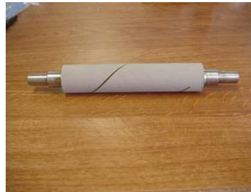
Trutz2334170G-R Trutzchler Cot w/ Arbor Repaired
