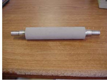
Trutz2334170-R Trutzchler Cot and Arbor Repaired
