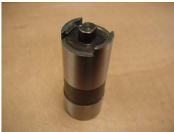
10117776R D35 End Bushing Repaired
