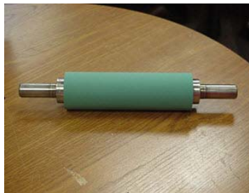
REIT2615038-J470R Rieter Cot and Arbor Repaired
