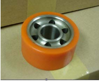
T-1692-420-008 Conveyor Pulley
